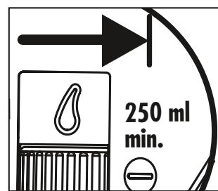
Set the spraying volume regulation (25) to "min". Start spraying operation for 2-3 seconds and moisturise microfibre pad (white). Drenching the surface has to be avoided because it may be that the edge areas of parquet or floor elements are not adequately protected against moisture.
