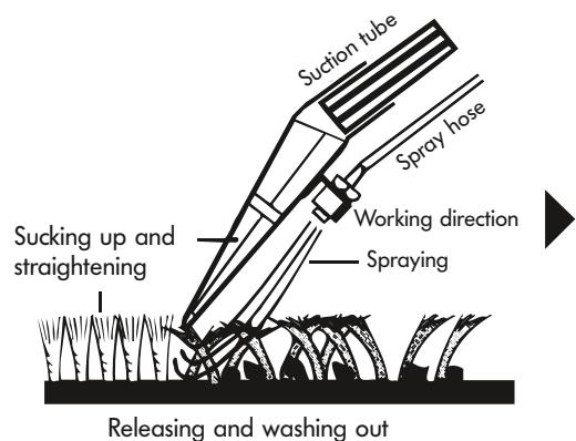
Press the lever on the shut-off valve (24) until cleaning liquid escapes. Draw the nozzle straight across the carpet and press it down at the same time. The spraying volume can be set as required by means of the little hand wheel on the handle. Release the lever to stop spraying at the end of one run or when stopping work. When the sprayed liquid has been sucked up, lift the nozzle and begin a new run but overlap slightly. In this way you can clean the entire area section by section.
