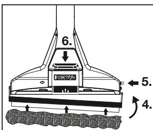
To remove the fold back hard floor adapter from the carpet spraying nozzle, pull the slide upwards and then press the red bolt on the nozzle towards the inside. Release the hard floor adapter from its hinge and remove.
